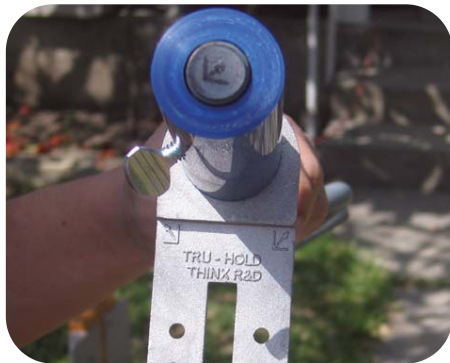
5 Adjust the required direction and height and screw the thumb screw to hold the hardware
