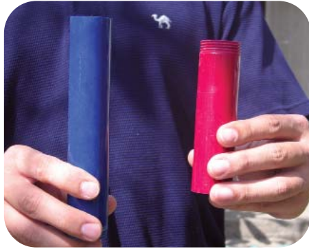
1 Choose the right color-coded tube for the size of the hardware.
