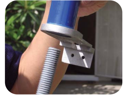
4 Slide the hardware into the opening on the bottom of the tube
